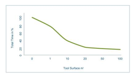
Compared to conventional tooling resins, the Polylite<sup>®</sup> Low Profile Tooling System allows manufacturing time to be reduced by up to 80% (depending on the tool surface involved).
