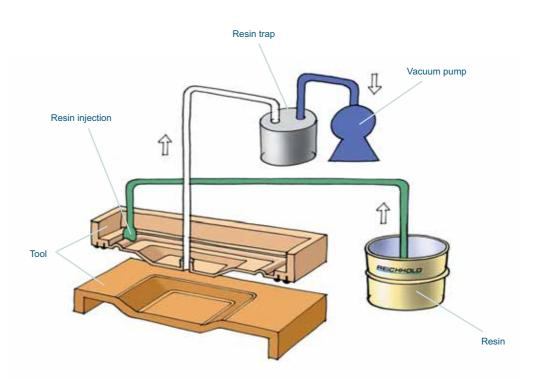
Vacuum Foil Infusion and Resin Transfer Moulding processes are widely used in the composites industry for manufacturing high quality components. These processes typically consist of the following steps:
