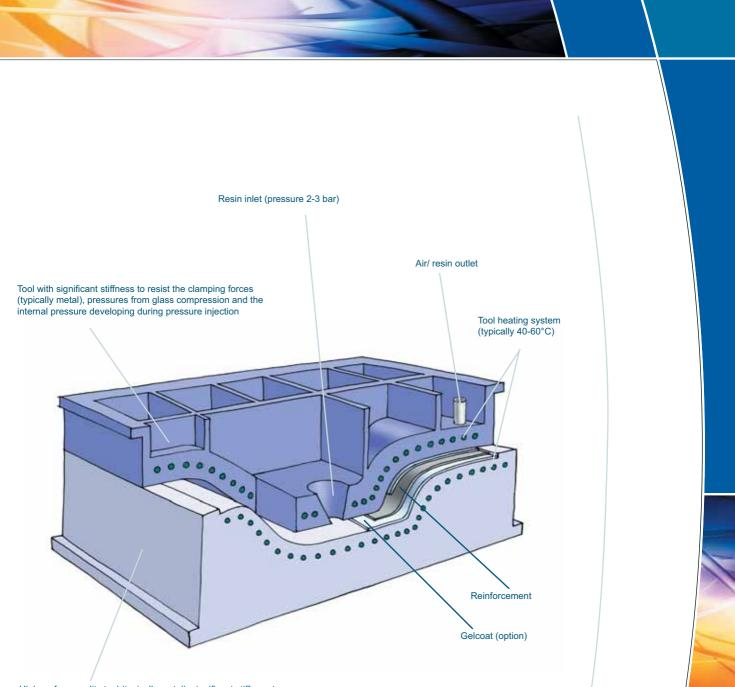
High surface quality tool (typically metal), significant stiffness to resist clamping forces, pressures from glass compression and pressure developing during injection
