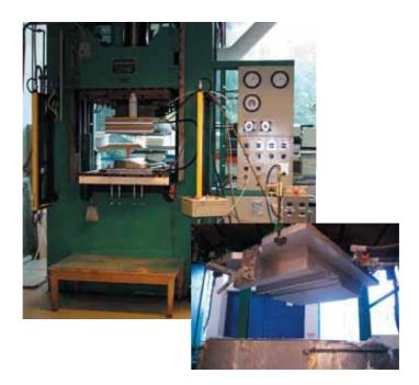
In this system the resin is forced into the mould by applying pressure. Usually heavy tooling is required on both male and female halves of the mould tool in order to resist the pressure generated during injection and to maintain dimensional consistency.
