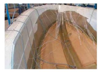
On a mould prepared with gelcoat, the dry reinforcement is sealed with a flexible transparent foil by vacuum. A special low viscosity injection resin is injected through a vacuum port and resin feed lines (e.g. bleeders).
