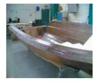
The process requires a rigid female mould and a semi-rigid male top mould. The mould closure is obtained by applying vacuum aided by simple clamping mechanisms.
