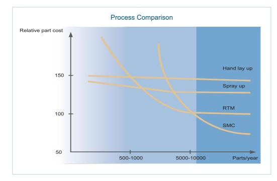
The cost break-even point between the processes will be dependent on several parameters as indicated above, so this graph represents only an indication of system cost.
