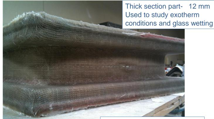
Glass wetting acceptable throughout entire composite part Deep vertical draw sections to ensure proper resin flow rates
